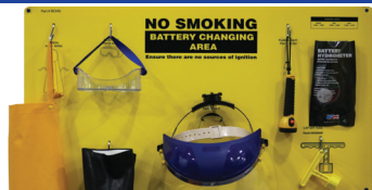
Forklift Battery PPE Board
